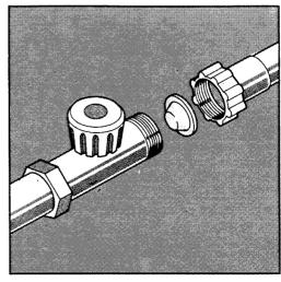
If only a cold water supply is available, connect the two hoses to a cold water outlet by means of a "Y" connection piece.
